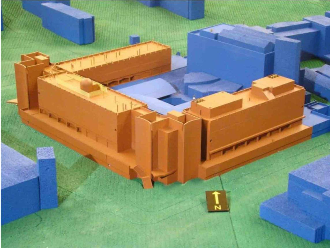
**Three-dimensional wind modeling of the complex helped architects better understand stack heights and other factors that would affect the facility during and after construction.** *(Courtesy of Goody Clancy)*
