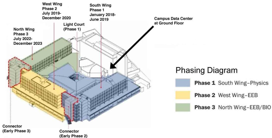
**This diagram shows the phased renovation of the Gant Science Complex at the University of Connecticut. When finished, the building will house physics, ecology, and evolutionary biology (EEB), in addition to other biology labs and teaching spaces. (Courtesy of Goody Clancy)**
