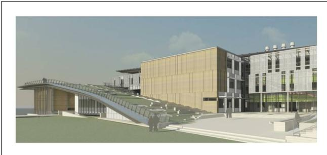
The proposed 'extensive' green roof, measuring approximately 14,000 sf, is mainly composed of a pre-grown, tray system with four inches of growing medium. The majority of the planting is comprised of sedum types, interspersed with varieties of California wildflowers, for areas not accessible to occupants.
